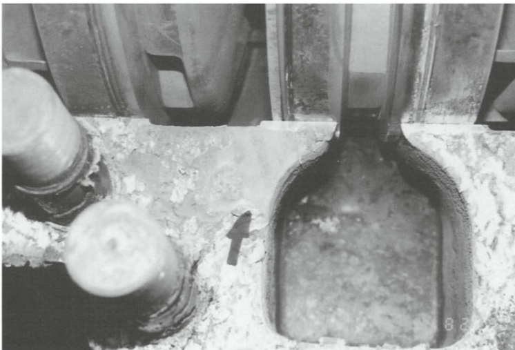
Figure 2.3 Internal leakage at joint - axially split pump multistage pump
