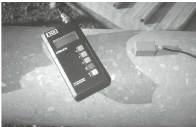
Figure 3.2 One type of ultrasonic flowmeter, with single transducer on pipe surface
