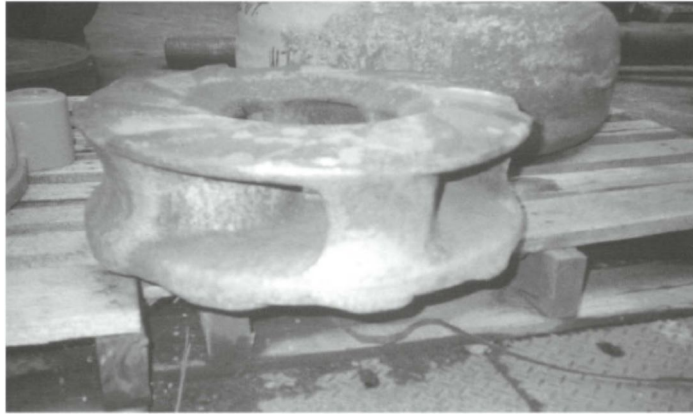
Figure 2.2 Impeller of ash slurry pump, showing general erosion
